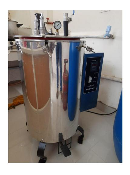
Microbiology laboratory generates microbial waste through regular laboratory activities and are treated by decontamination process in the specialized apparatus, Autoclave. The treated materials further added to the compost pits to convert to manure
